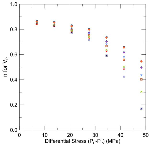
**Figure 6:** Example of empirical Biot coefficient for P-wave velocity for a sandstone sample as a function of differential pressure. Different symbols correspond to different pore pressures. In general, for a given differential stress,  $n$  decreases with increasing pore pressure.
