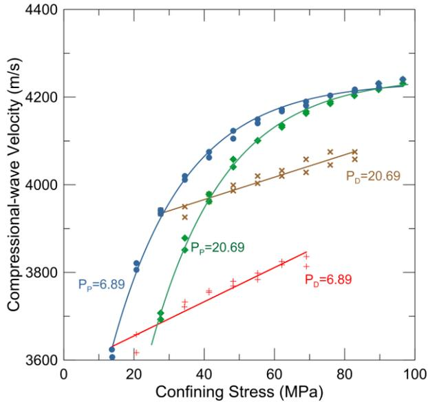
**Figure 5:** Example of compressional-wave velocity results for an arcose sandstone sample as a function of confining pressure with some constant pore pressure and constant differential pressure curves.
