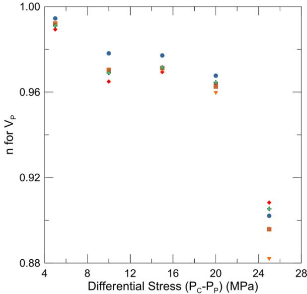
**Figure 8:** Example of empirical Biot coefficient  $n$  for P-wave velocity for a rudstone limestone sample as a function of differential stress. Different symbols correspond to different pore pressures values. In general, for a given differential stress, the coefficient decreases with increasing pore pressure.
