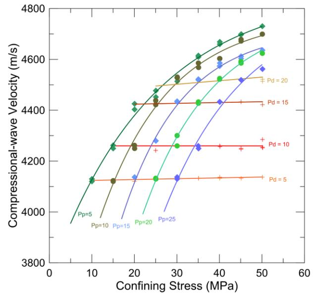
**Figure 7:** Example of compressional-wave velocity results for a limestone sample (rudstone) as a function of confining stress with some constant pore pressure and constant differential stress curves.
