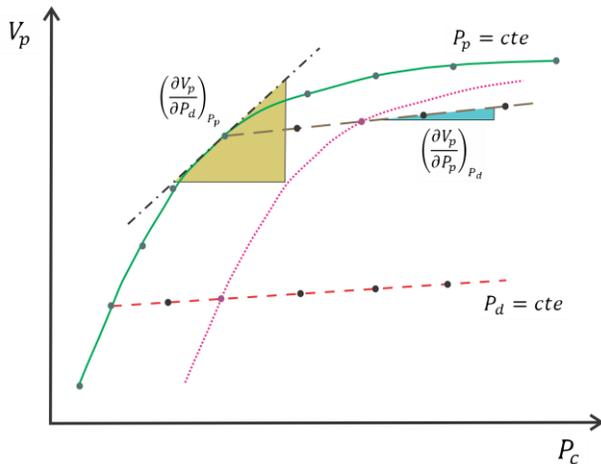
**Figure 1:** Schematic diagram of velocity versus confining pressure with the necessary partial derivatives for applying Todd and Simmons’ method. The continuous green curve correspond to velocity measurements obtained at different confining pressures with a particular pore pressure value, and the dotted pink curve to another pore pressure value. The dashed orange and brown straight lines correspond to velocity data collected at two particular differential pressure values.
